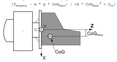
$J_{0z}$  is the moment of inertia around the Z axis at the center of gravity (CoG).
